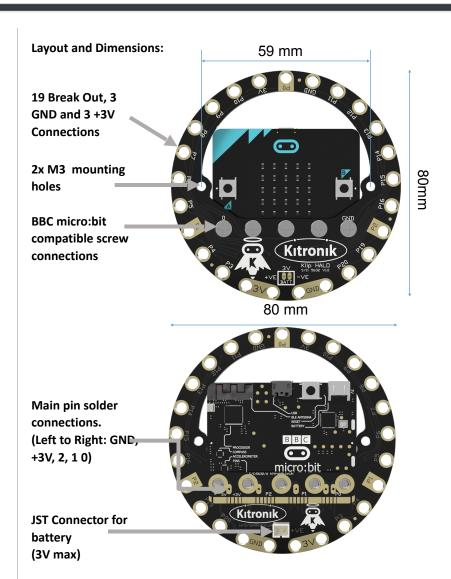
The Klip Halo board is 10mm thick (including micro:bit and bolts)
